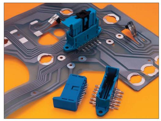
For decades, the automobile industry has used flexible foil circuits, among other applications, for instrument clusters and driver-side airbags. In order to implement these internal and external electrical connections, Tyco Electronics has an extensive range of contact systems in its repertoire.
